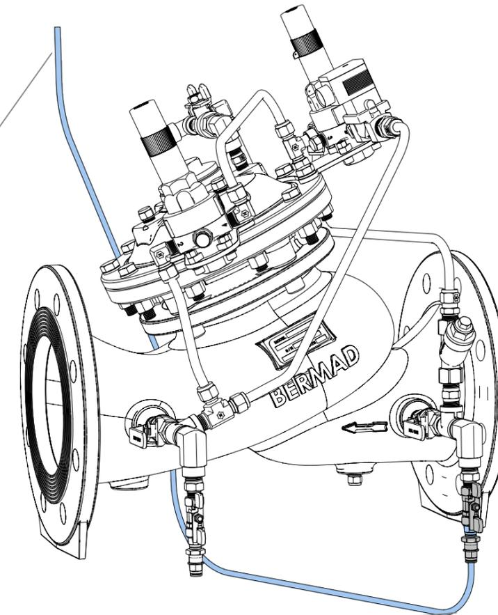
**3.** Connect the other end of the P1 tube to the P1 port on the controller
