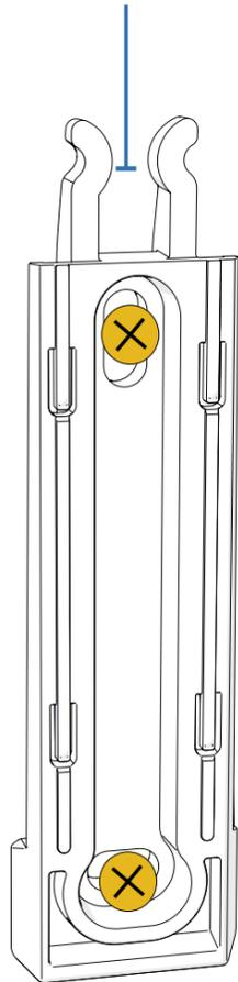
**2.** Connect the EPSILON data logger to the mounting bracket by sliding it into the groove
