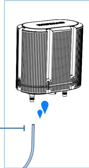
**1.** *Connect the P2 tube to the P2 fitting on the downstream outlet*
