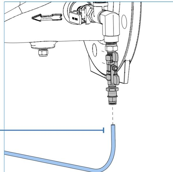
**2.** Open the cock valve and allow a slight flow of water to bleed the air from the P1 tube
