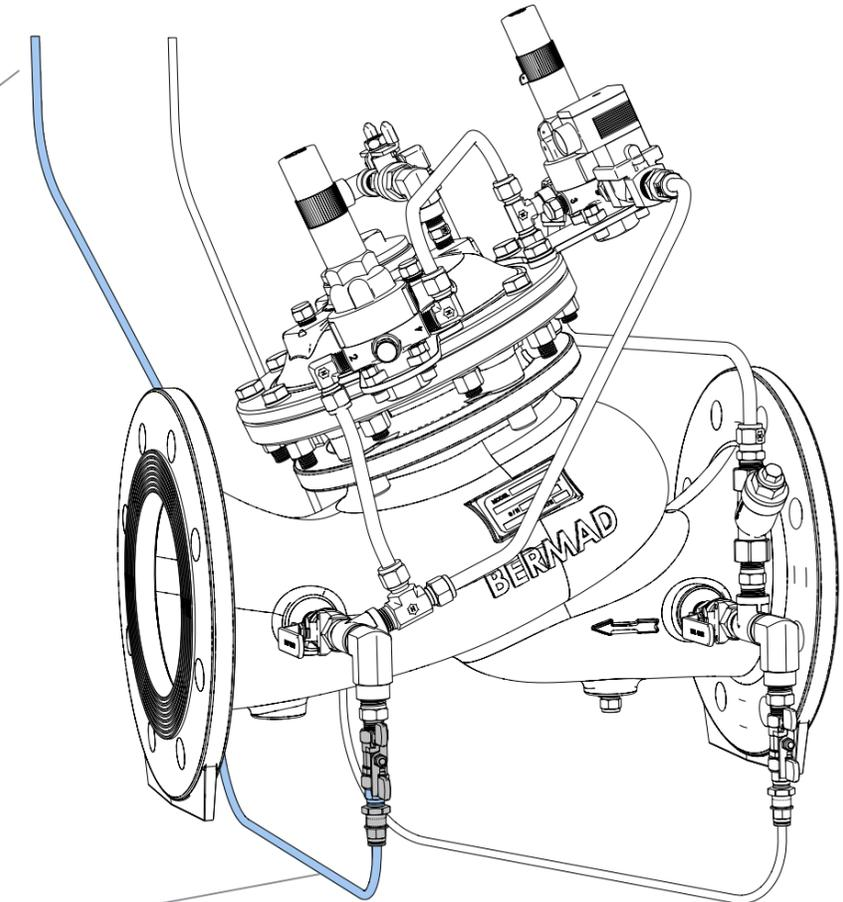
**3.** Connect the other end of the P2 tube to the P2 port on the controller
