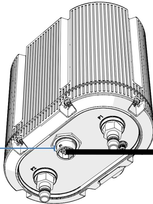
**2.** Connect the other end of the cable to the water meter
